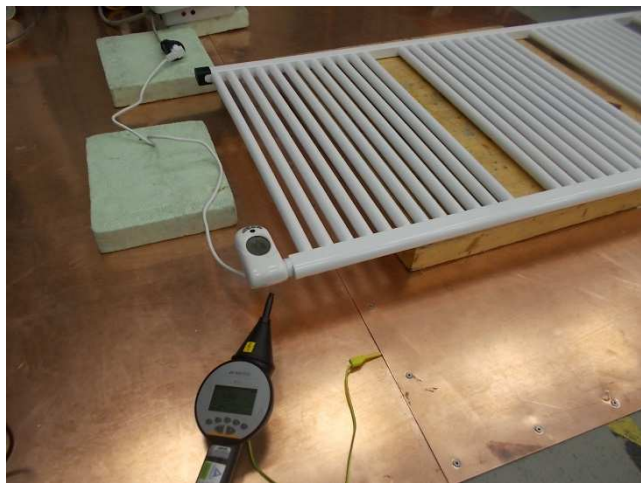
ESD test set-up
