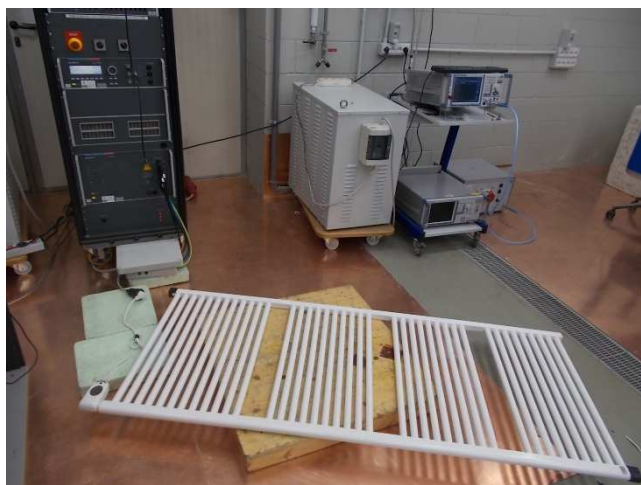
Burst/surge on AC input test set-up
