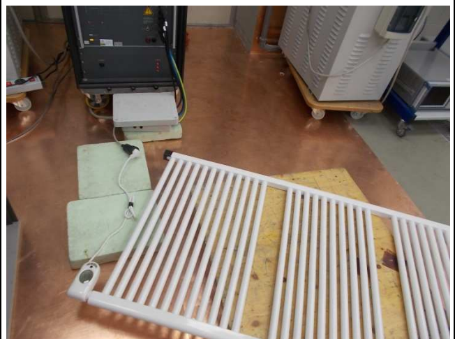
Burst/surge on AC input test set-up
