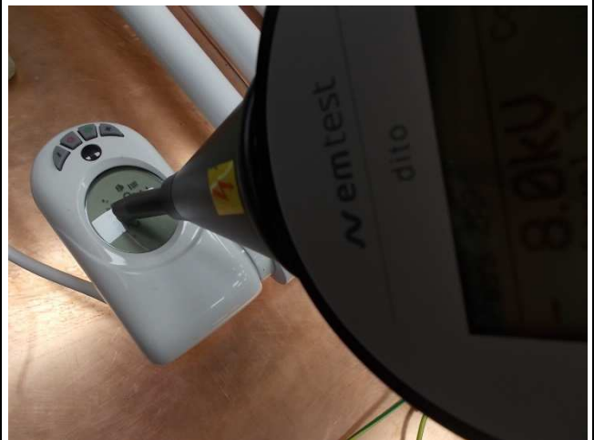
ESD test set-up
